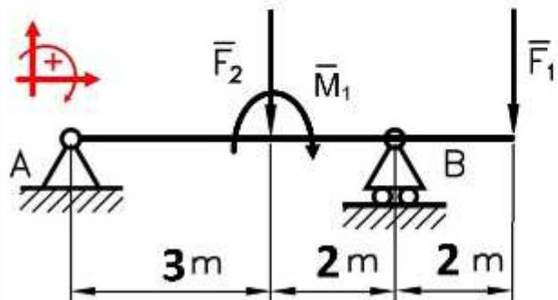
$$\begin{cases} \sum F_x = 0 \\ \sum F_y = 0 \rightarrow R_{AY} - F_1 - F_2 + R_{BY} = 0 \rightarrow R_{AY} - 7000 - 2000 + R_{BY} = 0 \rightarrow (\text{sostituendo}) \rightarrow R_{AY} = -3200 \text{ N} \\ \sum M_A = 0 \rightarrow F_1 \cdot 7 + F_2 \cdot 3 + M - R_{BY} \cdot 5 = 0 \rightarrow R_{BY} \cdot 5 = 7000 \cdot 7 + 2000 \cdot 3 + 6000 \rightarrow R_{BY} = 12200 \text{ N} \end{cases}$$
