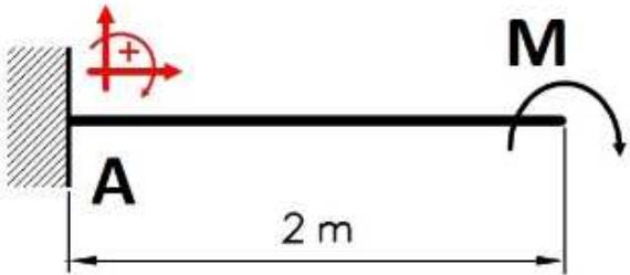
$$\left\{ \begin{array}{l} \sum F_x = 0 \\ \sum F_y = 0 \rightarrow R_{AY} = 0 \rightarrow R_{AY} = 0 \text{ N} \\ \sum M_A = 0 \rightarrow M + M_A = 0 \rightarrow 40 \text{ Nm} + M_A = 0 \rightarrow M_A = -40 \text{ Nm} \end{array} \right.$$
