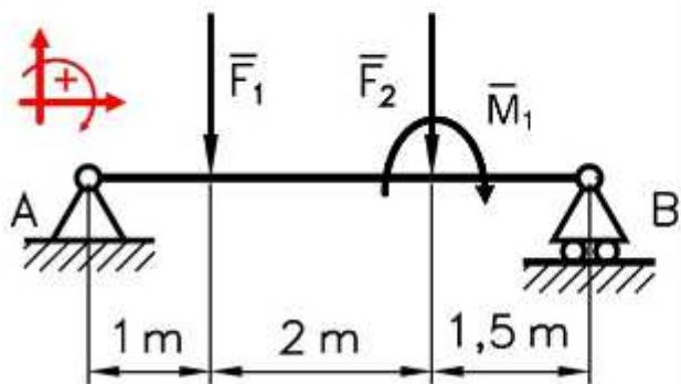
$$\begin{cases} \sum F_x = 0 \\ \sum F_y = 0 \rightarrow R_{AY} - F_1 - F_2 + R_{BY} = 0 \rightarrow R_{AY} - 7000 - 4000 + R_{BY} = 0 \rightarrow (\text{sostituendo}) \rightarrow R_{AY} = 6333 \text{ N} \\ \sum M_A = 0 \rightarrow F_1 \cdot 1 + F_2 \cdot 3 + M - R_{BY} \cdot 4,5 = 0 \rightarrow R_{BY} \cdot 4,5 = 7000 \cdot 1 + 4000 \cdot 3 + 2000 \rightarrow R_{BY} = 4667 \text{ N} \end{cases}$$
